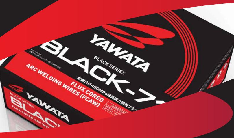
YAWATA BLACK-71 is a titania type flux cored arc welding wire for all position welding with CO2 shield gas. The wire is baked giving it the distinct black colour appearance. The baked wire has very good feedability, excellent anti-rust property and low fume generated.
